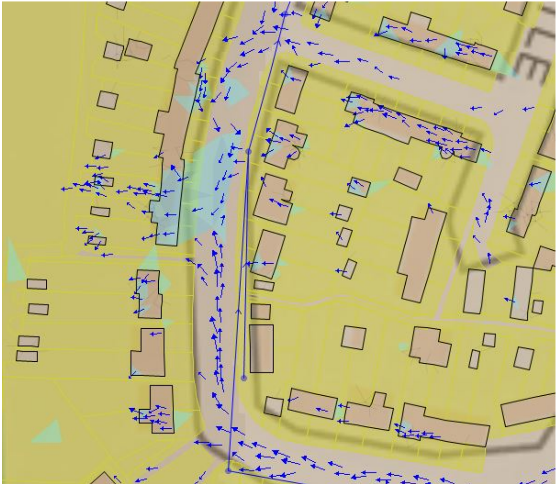
Figure 5-3: Surface water leaving the highway and flooding property along Thistle Grove
